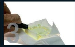
Remove excess colour using compressed air, while holding the work over a suitable piece of cellulose.
