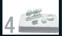
Dry on a firing tray under the drying lamp Zirkonlampe 250. It is recommended that the drying is carried out under an extraction hood or outdoors.
